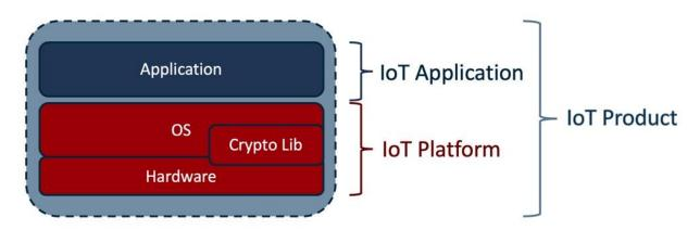
An IoT Platform, defined as Connected Platform in [SESIP], is the hardware/software providing an operating environment for an IoT Application. IoT Platforms parts can be developed and evaluated separately, for example by evaluating the cryptographic library, an OS, hardware, and then combining them. In terms of the Common Criteria, the IoT Platform (part) identified in the ST is our TOE.
