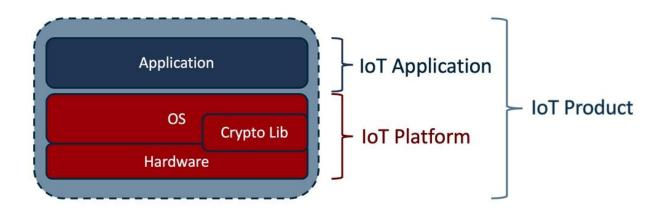
An **IoT Platform** is the hardware/software providing an operating environment for an IoT Application. IoT Platforms parts can be developed and evaluated separately, for example by evaluating the cryptographic library, an OS, hardware, and then combining them. In terms of the traditional Common Criteria, the IoT Platform (part) identified in the ST is our TOE.
