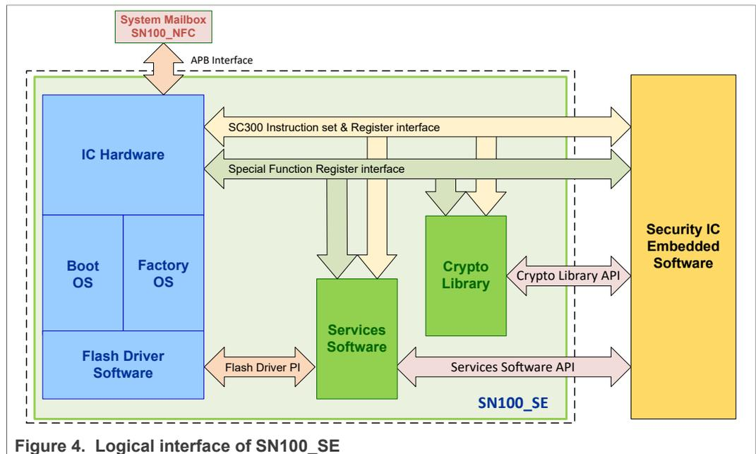
Figure 4. Logical interface of SN100\_SE
