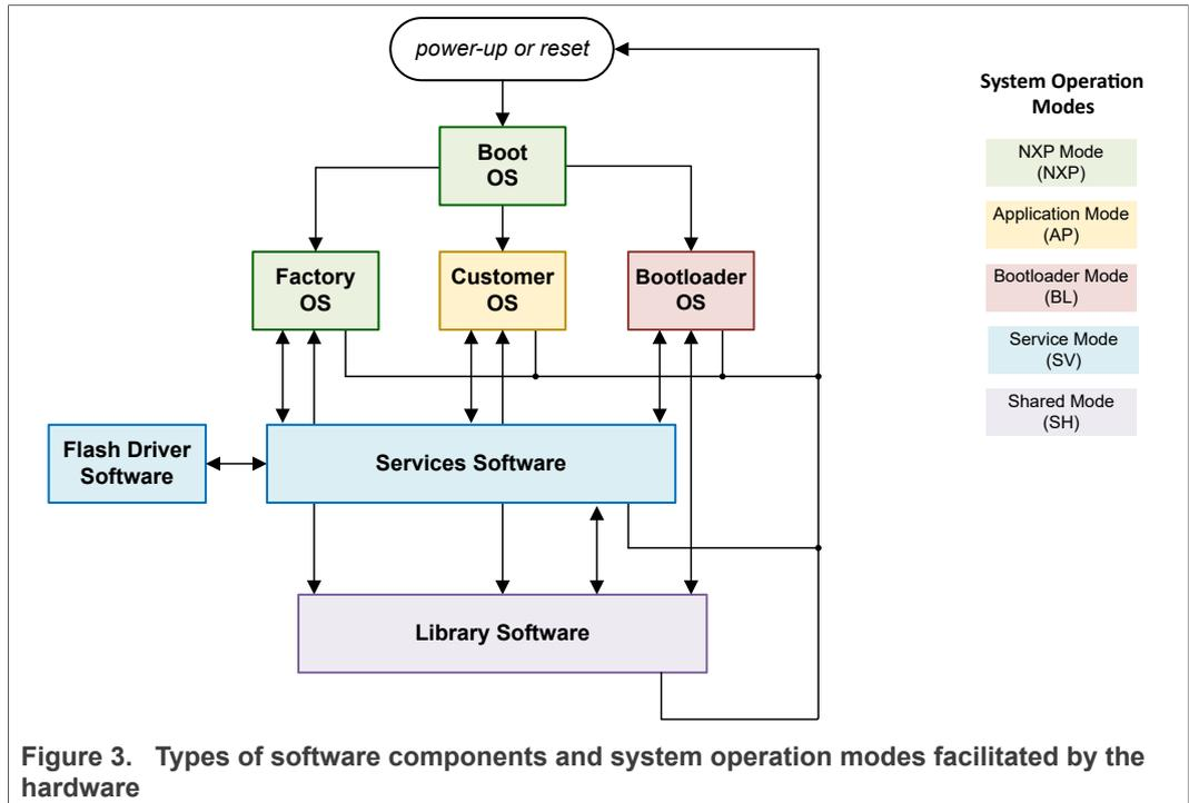
Figure 3. Types of software components and system operation modes facilitated by the hardware
