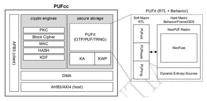
The hardware modules of PUFcc, including the Verilog RTL design and the hard-macro, are shown in the figure above. Note that the TOE hardware includes the Verilog RTL design and the behavioral model of the hard-macro on the FPGA board. That is, the behavioral model emulates the hard-macro by FPGA. Hence, only source code reviews of the hard-macro design will be performed, and any penetration testing on the protection provided by the hard-macro will be out of scope of this certification program.
