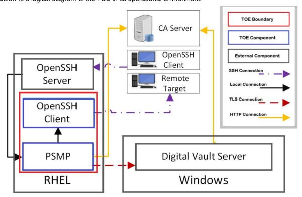
A user connects to PSMP by providing a target device, target user, Vault user, and Vault password, which are then relayed to the Digital Vault Server for verification. Once the user is verified, PSMP retrieves the target user's credentials to connect the user to the target device. While a user is connected to a target device and is performing activities in the privileged session, PSMP actively
