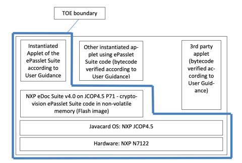
The whole applet code resides in the Flash memory; the applets providing these different configurations are instantiated into Flash memory. Multiple configurations (and hence support for different applications) can be present at the same time by instantiating multiple applets with their distinct configurations.
