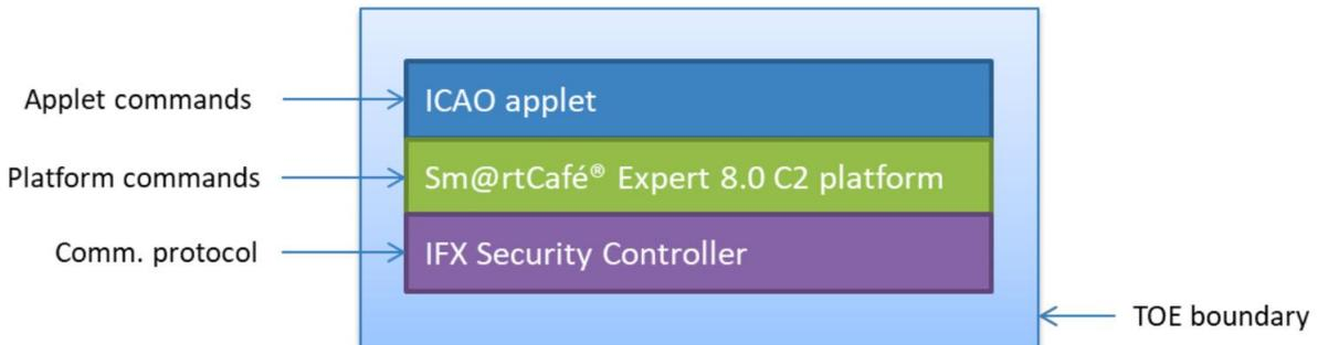
The TOE is an applet named ePass applet based on Sm@rtCafé® Expert 8.0 C2 platform, which is used as an ICAO eMRTD, which can be configured to support the different authentication mechanisms.
